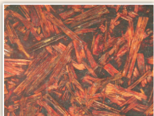
Particle board made of Parthenium
